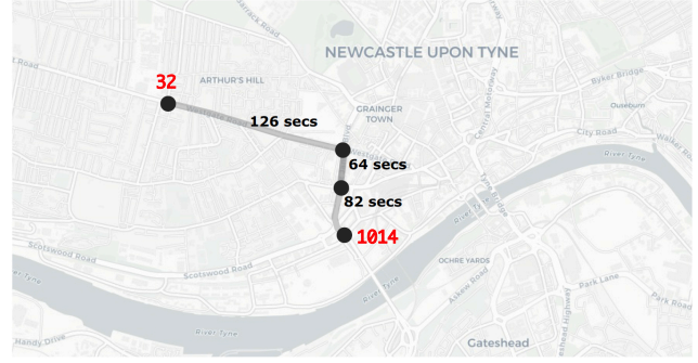
Figure 4: Example of a trip of degree 4. On the left side the corresponding data table is shown. The u_{th} trip of each vehicle is given by the variable Trip , whereas the i_{th} sighting is given by variable Sighting . The variable JourneyTime gives the travel time from the previous to current sighting. Lastly, the variable TripId represents the unique sequence of cameras that describes the trip. This allows trips to be grouped and summarised not only in terms of their origins and destination, but also routes. On the right side, the same trip is plotted on a map. The circles represent camera locations whereas the lines represent the fastest driving routes between sightings rather than the true route taken by the vehicle. Even though no routing information is available for each consecutive pair of sightings, the observed journey times can be compared against the distribution of collective journey times to rank the set of most likely routes chosen (which can be determined for instance by Stochastic User Equilibrium [3]).
